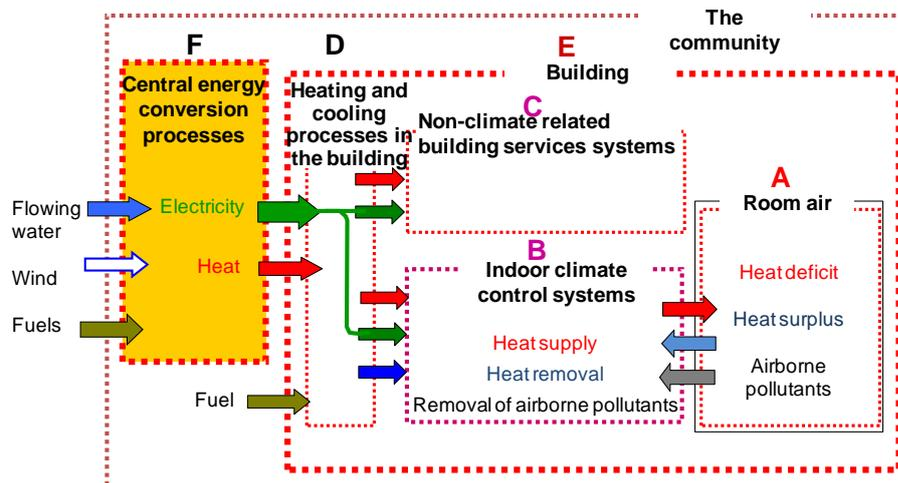
**Figure 1.** System boundaries that can be applied when analysing the energy behaviour of a building.
